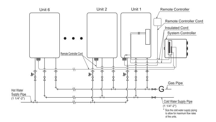
• Insulate or apply heating materials to both the cold water supply piping and the hot water supply piping to prevent freezing during cold weather and to prevent heat loss through the piping.
