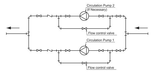
Adjust the pump flow with the flow control valves. If multiple pumps are used, control the flow of each pump with separate valves.
