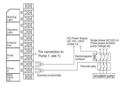
\* Do not connect both of pumps 1 and 2 to the same terminal blocks.
